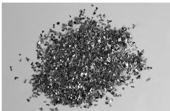
Fig. 1. Morphology of powder prepared by centrifugal atomization.
